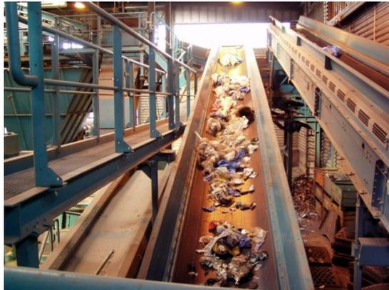
Ashes automatically being carried by conveyors in a solid-waste treatment
