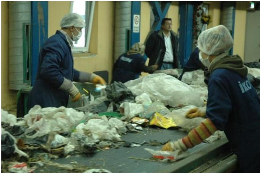
Recycle process in a solid-waste treatment plant
